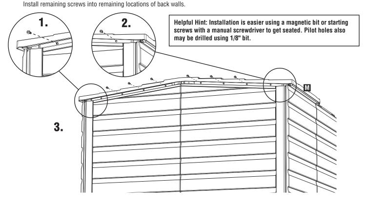
From inside the shed, install four **Screws (AA)** into the roof, two on each side wall.
